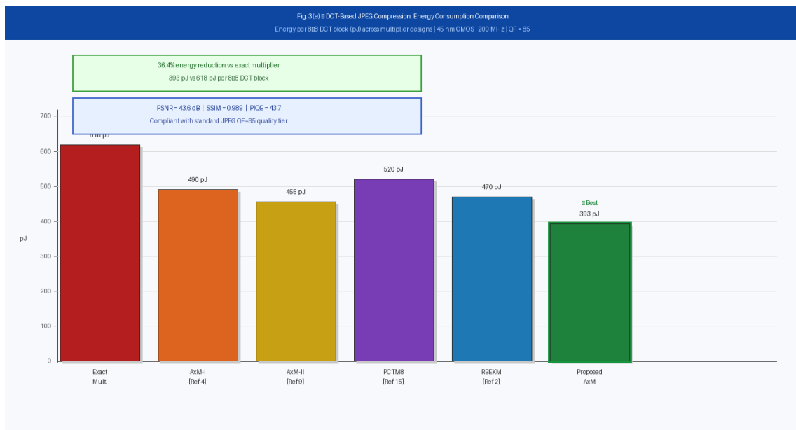
Fig. 3(e) — DCT Energy Consumption Comparison: Proposed AxM achieves 393 pJ (36.4% reduction vs. exact)
