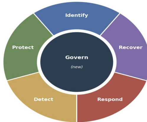
Govern overlays all five existing functions: org context, risk strategy, supply chain, oversight.
